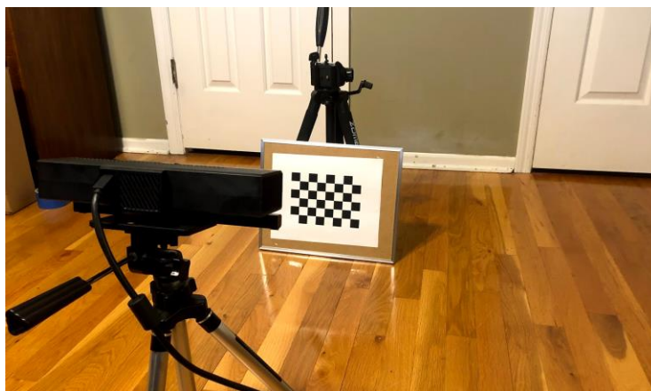
Figure 5: Physical Setup of Kinect and Calibration Photo
