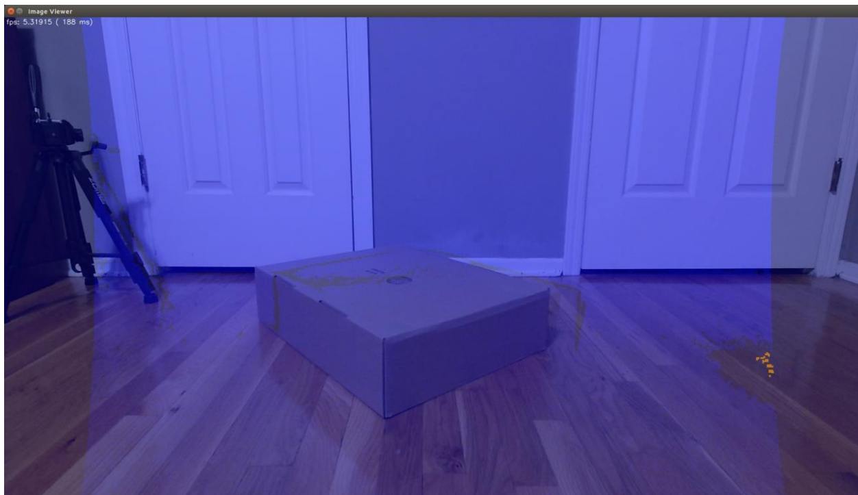
Figure 2: Pre-Calibration Photo – RGB and IR Sensor are Not Aligned
